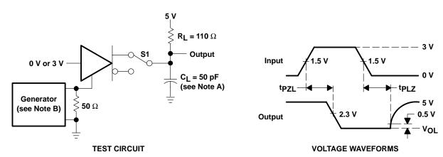
NOTES: A. Cl includes probe and jig capacitance.
