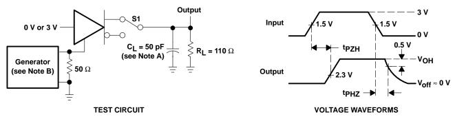
NOTES: A. CL includes probe and jig capacitance.
