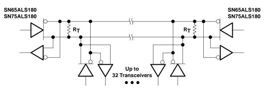
NOTE A: The line should terminate at both ends in its characteristic impedance ( $R_T = Z_O$ ). Stub lengths off the main line should be kept as short as possible.
