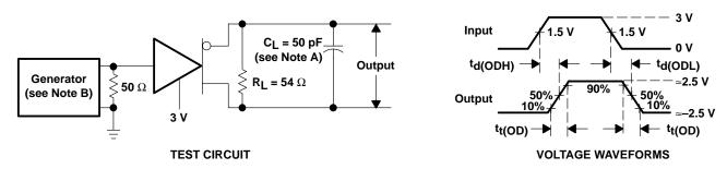
NOTES: A. CL includes probe and jig capacitance.
