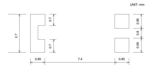
Note: Please make sure that there is no electric wire line under SSP-T5 on the circuit board.
