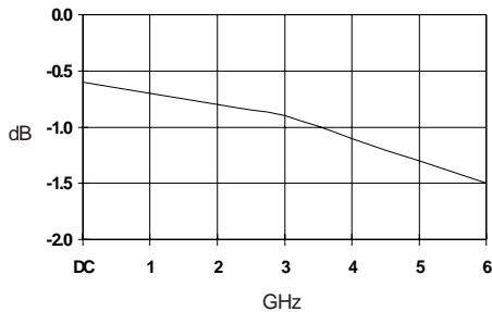
Insertion Loss vs. Frequency V Control = -5 V
