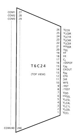
Note: The above diagram shows the pin configuration of the LSI chip; it does not show the configuration of the tape carrier package.
