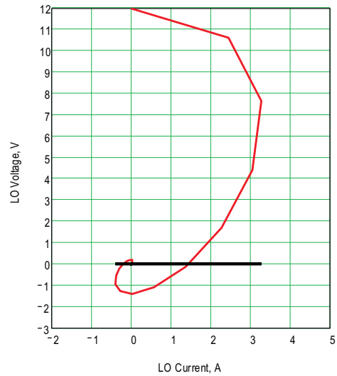
Figure 25. Turn-Off Voltage and Current Switching Diagram
