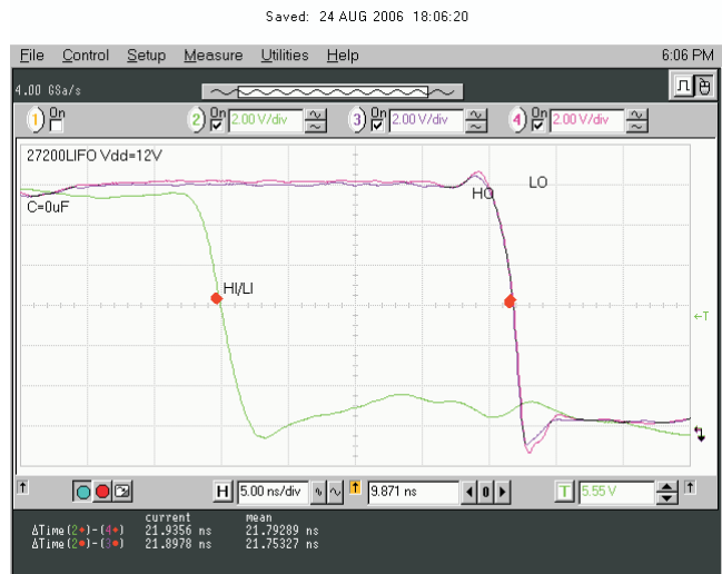
Figure 32. V_{LO} and V_{HO} Falling Edge Delay Matching
