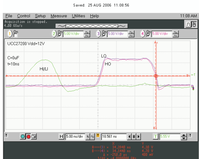
Figure 34. 10-ns Input Pulse Delay Matching
