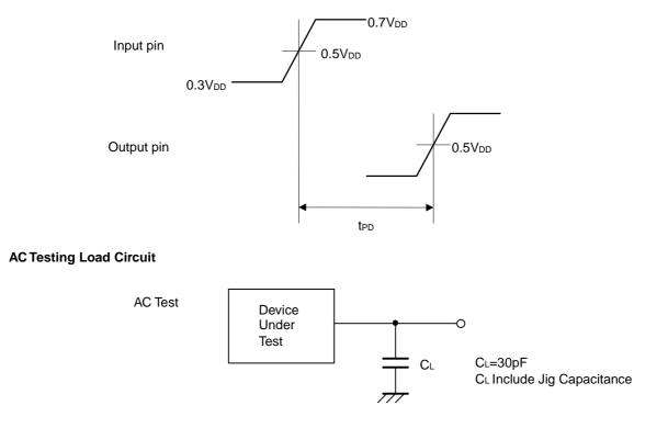
**Remark** In case of CL=50pF, the operating condition changes to  $T_A = 0$  to +70 °C.
