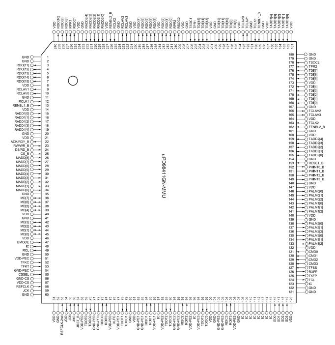
Remark1. IC: internal connect pin. Leave the IC pins open.
