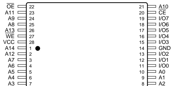
28-Pin TSOP (Standard)
