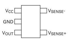
The ZXCT1051 provides a fixed gain of 10 thereby removing the need for an additional resistor.
