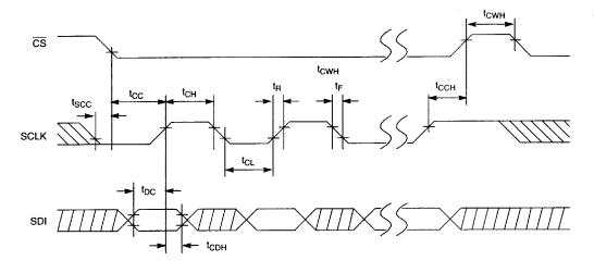
**Note:** SCLK can be either high or low when  $\overline{CS}$  is taken low.
