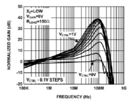
FIGURE 3. GAIN vs FREQUENCY FOR VARIOUS VCTRL
