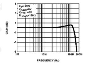
FIGURE 1. FREQUENCY RESPONSE OF ALL CHANNELS
