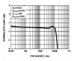
FIGURE 2. GAIN vs FREQUENCY ALL CHANNELS
