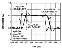
FIGURE 22. PULSE RESPONSE FOR VARIOUS CABLE LENGTHS
