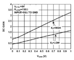
FIGURE 10. DC GAIN vs VGAIN
