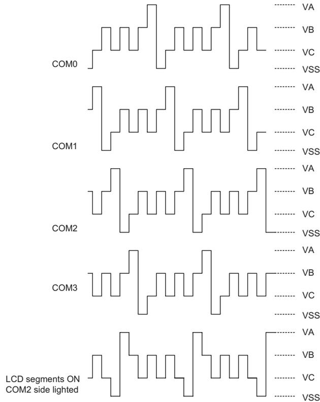
Note: 1/4 duty, 1/3 bias, C type: "VA" 3/2 VLCD, "VB" VLCD, "VC" 1/2 VLCD
