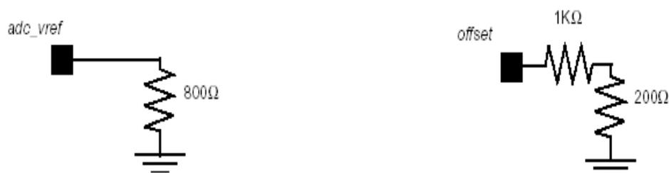
Figure 4. Equivalent Circuits For *adc\_ref* and *offset* pins
