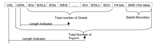
The diagram below shows the layout of the User-Data for eight bit SM data.
