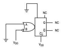
Figure 14. Connection of Unused Sections
