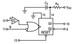
$R_X$  AND  $C_X$  ARE EXTERNAL COMPONENTS.  $V_{DD}$  = PIN 16  $V_{SS}$  = PIN 8, PIN 1, PIN 15
