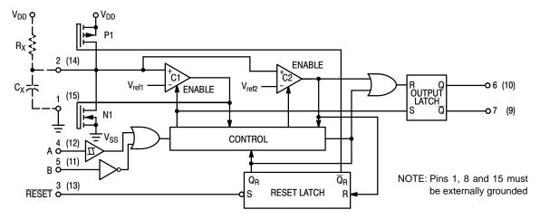
Figure 1. Logic Diagram (1/2 of Devlce Shown)
