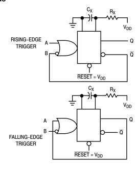
Figure 13. Non-Retriggerable Monostables Circuitry
