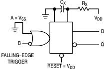
Figure 12. Retriggerable Monostables Circuitry
