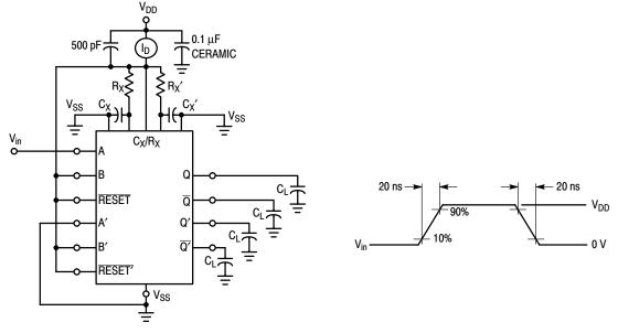
Figure 2. Power Dissipation Test Circuit and Waveforms
