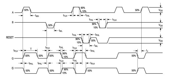
Figure 4. Switching Test Waveforms
