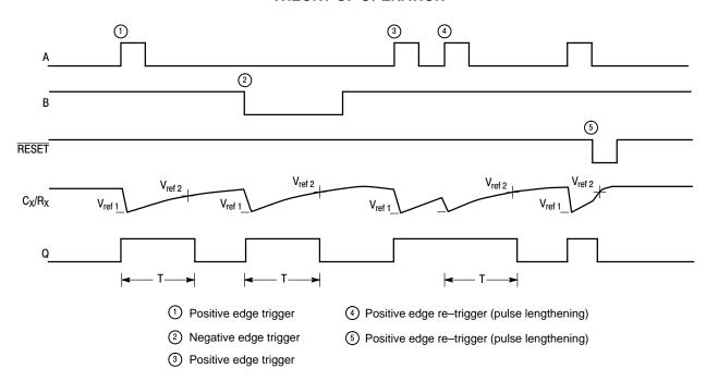
Figure 10. Timing Operation
