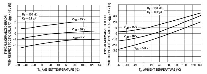
Figure 8. Typical Error of Pulse Width Equation versus Temperature
