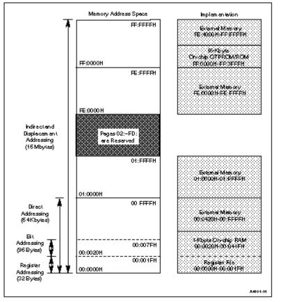
Figure 3. 8XC251SB Memory Mapping
