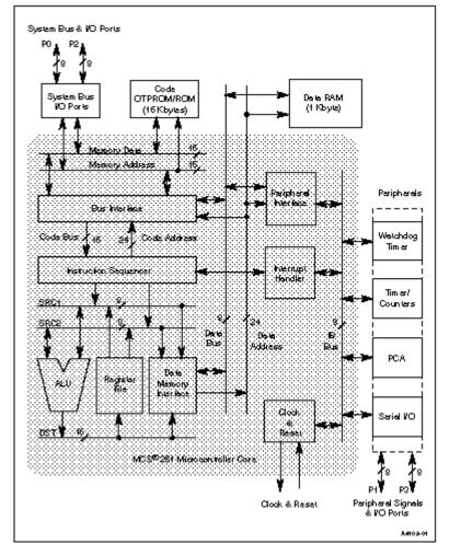
Figure 1. 8XC251SB Functional Block Diagram
