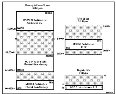
Figure 2. MCS<sup>®</sup> 51 Memory Mapping in 8XC251SB
