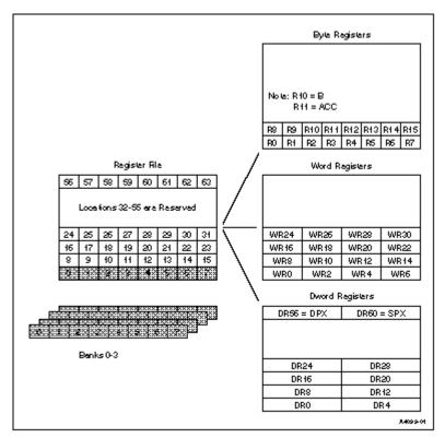
Figure 4. 8XC251SB Register File
